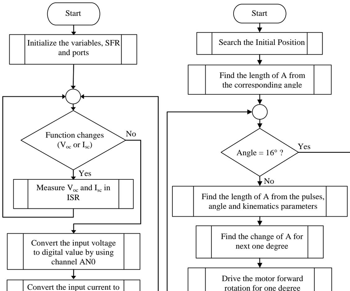
Figure 7. Flowchart of control program for solar power measuring section
