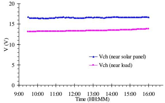
Figure 10. Voltage versus time graph with tracking
