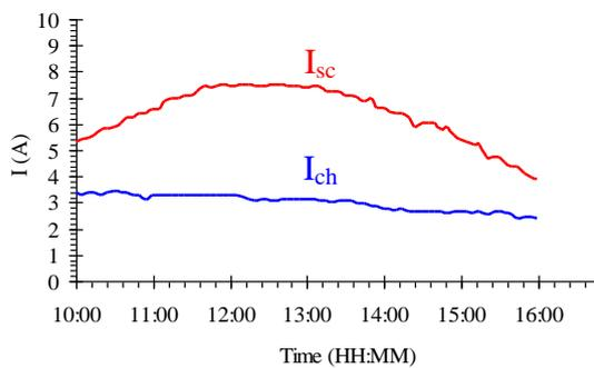
Figure 11. Current versus time graph without tracking
